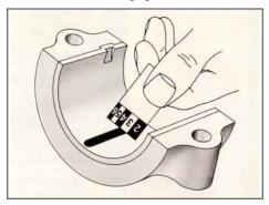
For most applications .00075 to .0010" (three quarters to one thousandth of an inch) of clearance per inch of shaft diameter is a reasonable starting point. For example, a 2.000" shaft diameter
