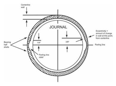
For these reasons, bearing clearances are specified as "vertical clearance" and must be measured at 90 degrees to the split line. The best method of measurement is with a dial bore gage that measures the bearing inside iameter when the bearings are installed at the specified torque without the shaft in place. Measurements should be taken at front, center, and rear of each bearing position. Another common method of checking clearance is through the use of CLEVITE 77® Plastigage®.
