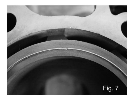
9. Complete the o-ring install by repeating these steps on all cylinders. You are now ready for your head install. (Be careful not to set anything on the deck surface that may ding, scratch or harm the o-ring wire in any way!)
